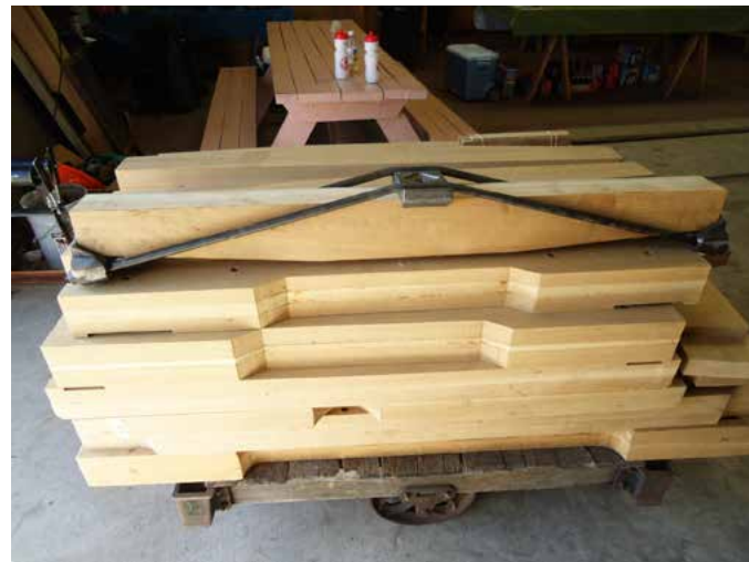
Wood parts for 470 trucks with one set of newly cast brake beam truss rod parts in place
