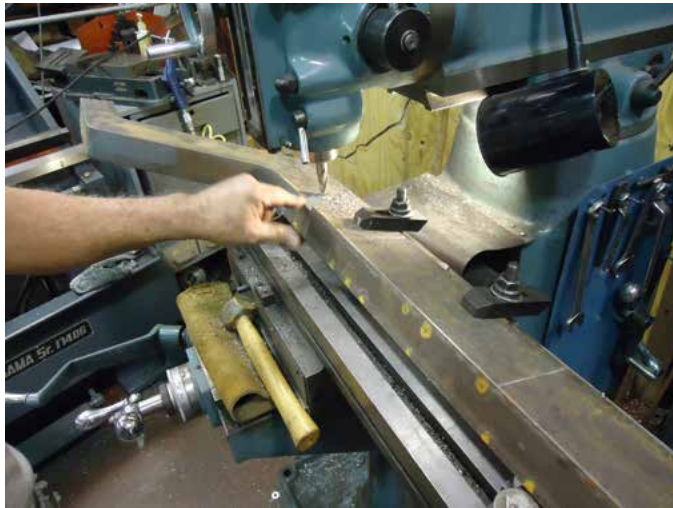
Machining an equalizer bar for the RPO in the CRF
