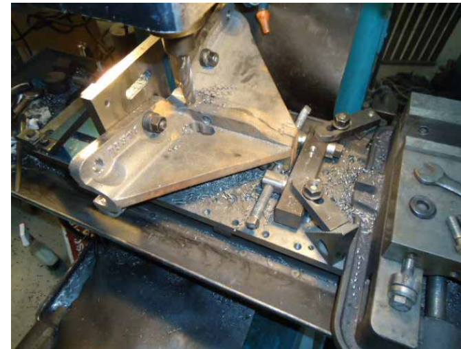
A pair of inside corner brackets for composite trucks being machined
