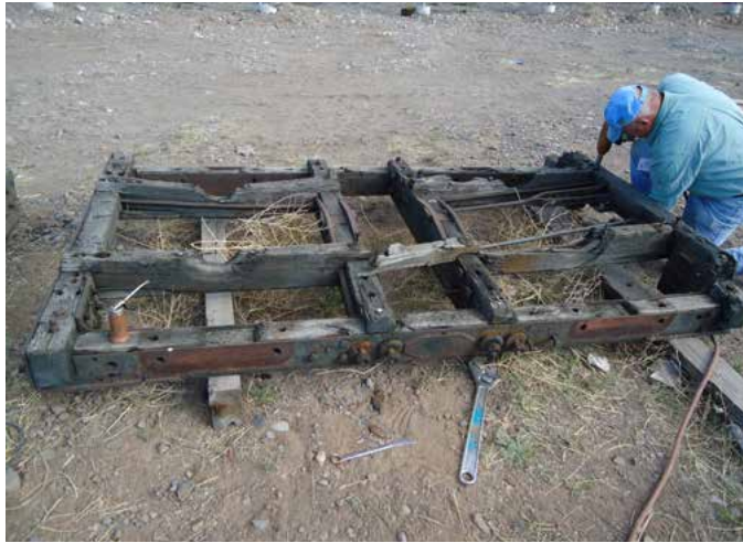
Disassembling a composite truck carcass for parts and information.
