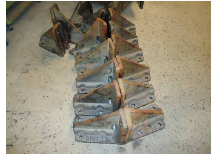
Interior corner plates for composite trucks after machining. A composite truck is one made of wood and metal
