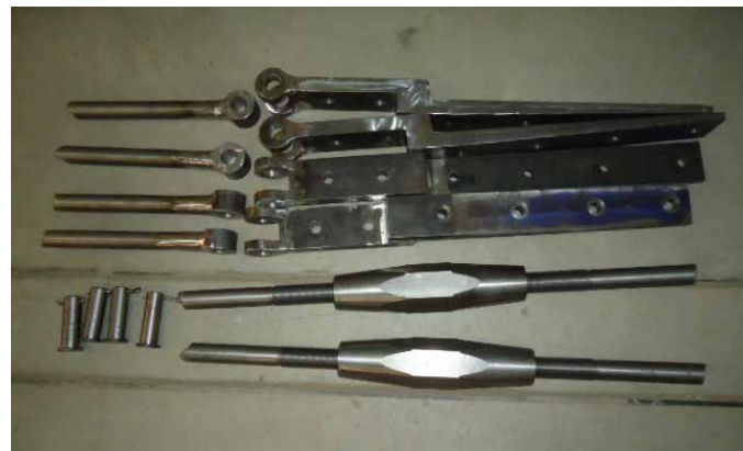
Fabricated ends and turn buckles for 470 truss rods
