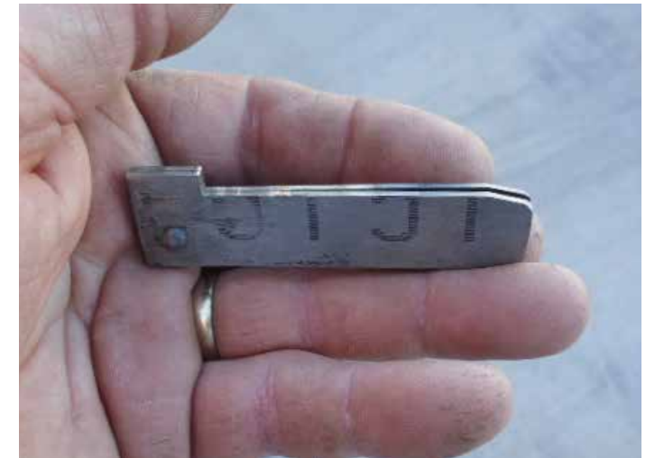
This is a type of cotter pin frequently used by the D&RGW; cutting the slot is a real pain.
