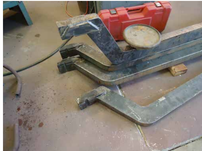
Completed equalizer bars for the RPO. The Friends had the 2" thick bars CNC torch cut but then we welded on the end tabs and machined the end grooves and slots to retain the spring pockets (one shown in place)
