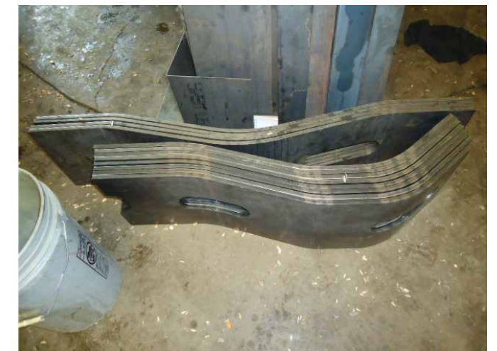
Parts for a flying bolster ready for welding
