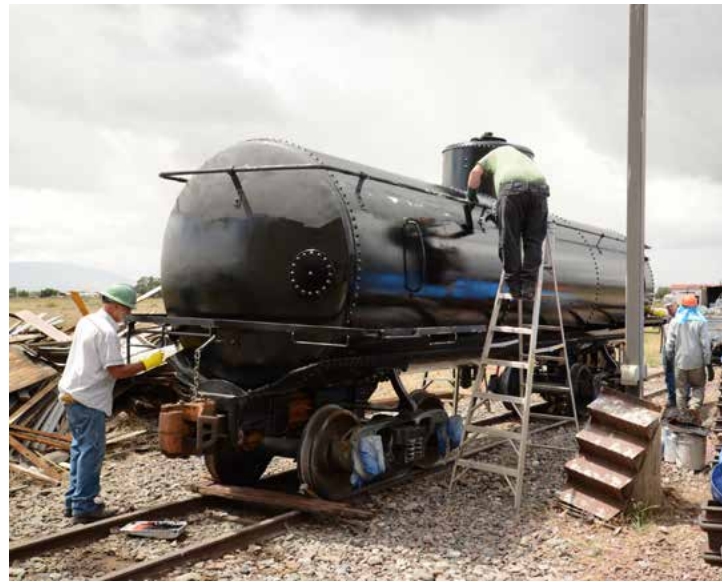
TL Don Stewart and team hard at it in Antonito painting one of the frameless tank cars.
