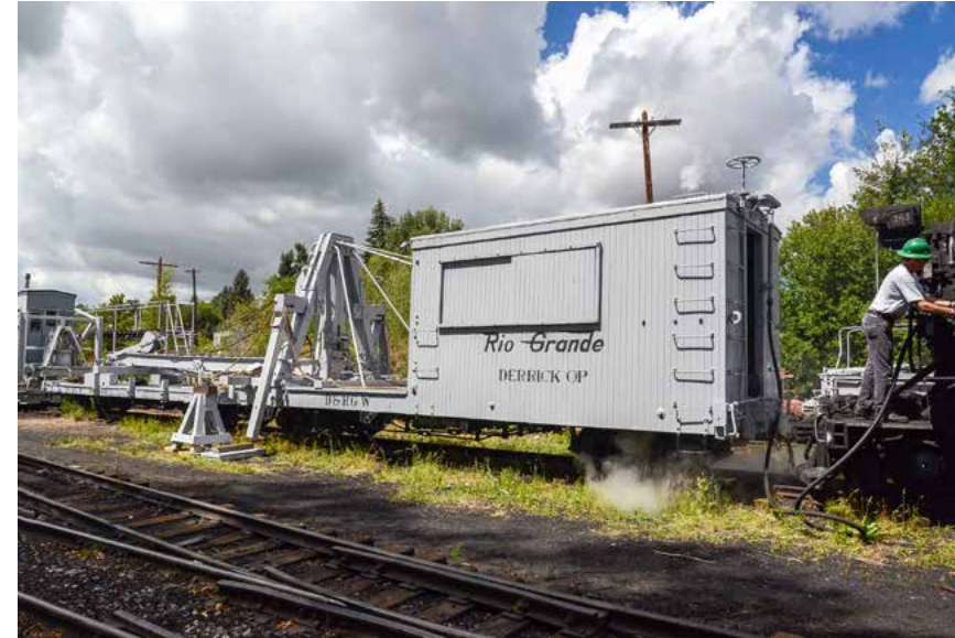
One of the highlights of Session "F" was restored derrick OP being connected to steam (engine 484) for the first time in about 40 years.
