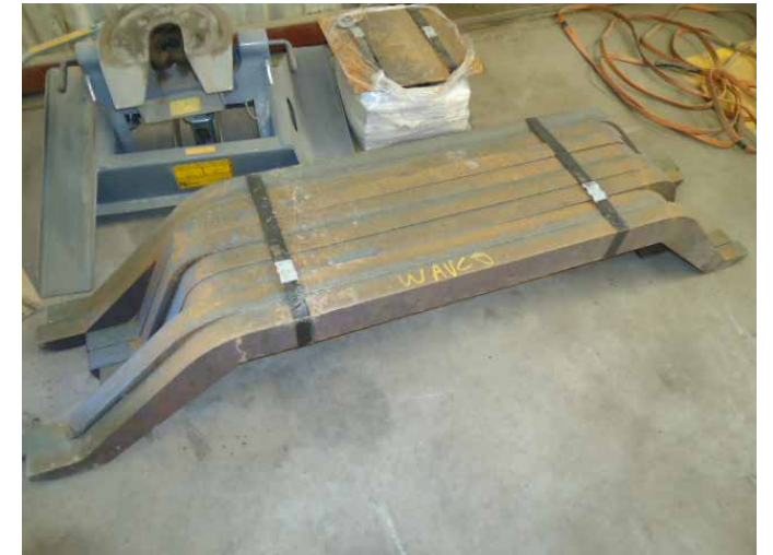
A bundle of torch cut equalizer bars ready for machining; these are for 470 and the RPO
