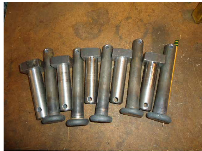
The brake linkages require lots of pins to hold them together - these are a few examples
