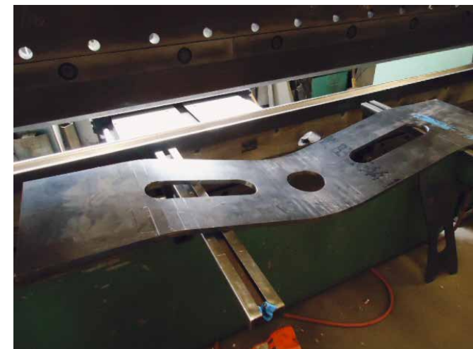
Bottom plate for flying bolster being formed at a local shop
