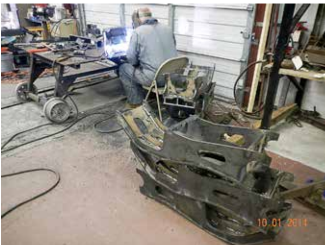
Flying Bolster halves - 8 completed waiting to be ground.
