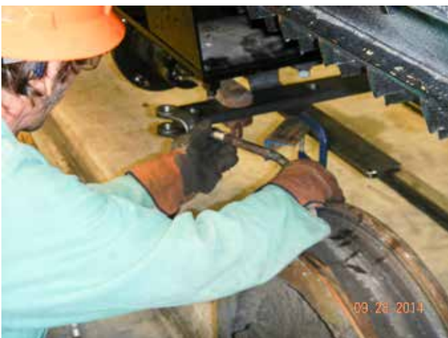
New rigging for the tank cars is a matter of trial and error.
