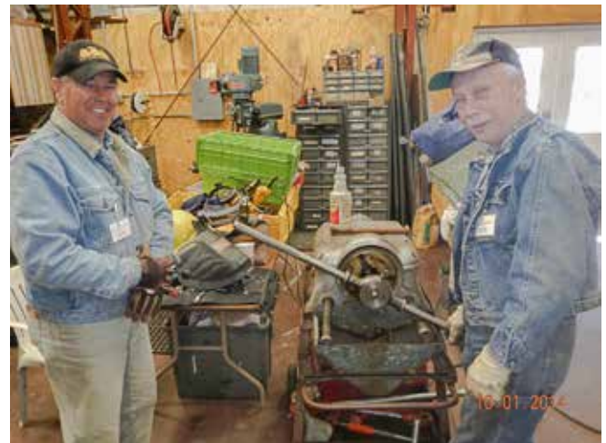
Doug Joslyn and Kevin Corwin threading air line pipe.
