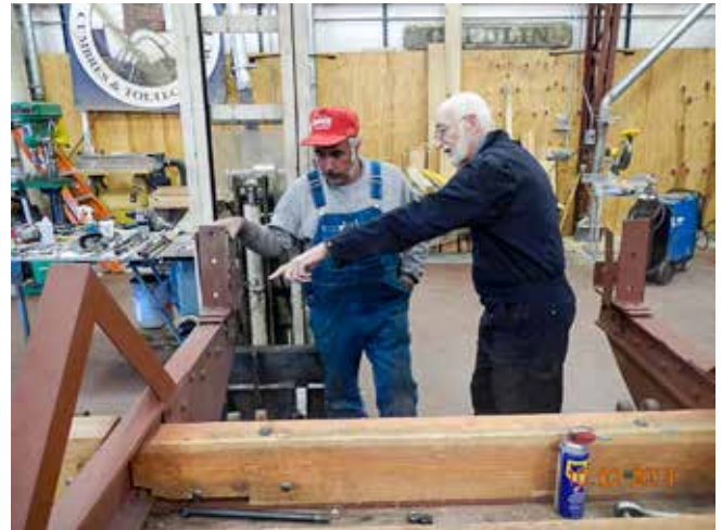
Marvin Casias and Warren Ringer checking for cracks. None found.
