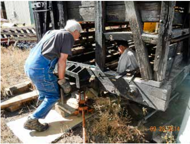
Kevin Corwin and William Horker installing a coupler on A end of Long Stock car 5995.
