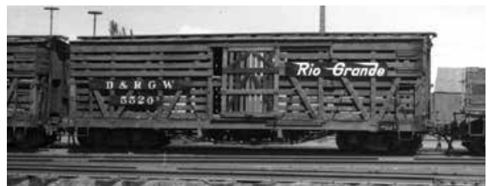
30-foot 5500-Series D&RGW Stock Car 5520, built in 1904 and rebuilt in 1926. Look closely and you will see the small “D” following the number. FCTS BRK03-193
