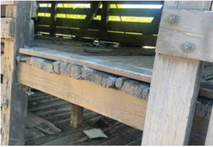
Double-deck sheep cars were a simple affair with a platform half-way up the interior and a split door. You can see the support mortised into the door frame and a threshold on top of the floor boards to prevent damage to both the car and the cattle. A simple post supported the center, placed upon a piece of burlap, tin, wool or wood to keep the wet floor from rotting under the post. Photo by Tom Stewart
