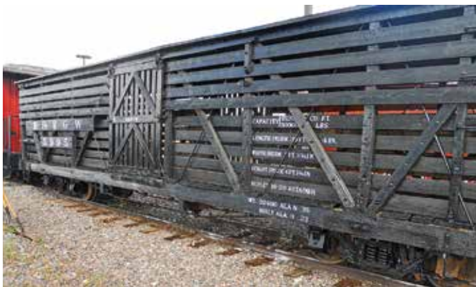
Stock Car 5995, a 34-foot 5900-Series D&RGW Stock Car, built in 1916, was restored by the Friends of the C&TS. 5995 is the only surviving 5900-Series Stock Car. Photo by Tom Stewart
