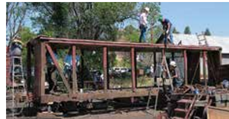
Converting P-Box 207 to a Rider Box Car.
