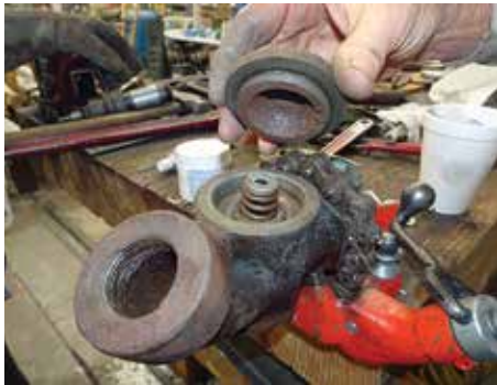
The angle cock, the air valve at the end of the car, came from a scrapped car. It needed some cleaning before installation.
