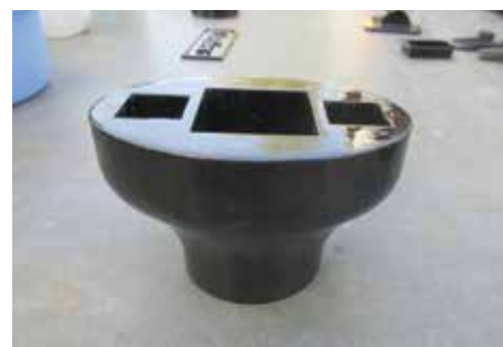
The finished berth stop pattern.
