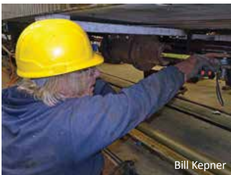
Bill checks the length of travel on the piston of the brake cylinder.
