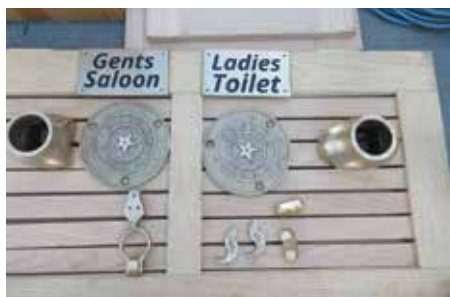
Signage, builder's plates and many tiny pieces were cast as well.
