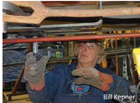
There are a lot of components that make up the brake linkage under the car that must work together.
