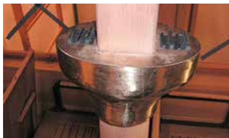
One of the finished berth stop blocks in place in Car 470.
