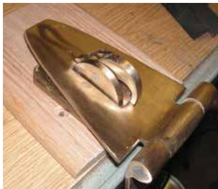
The combined multi-piece latch and hinged clasp keeps stowage of the upper berth securely in place.
