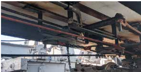
More than air: air brakes include a series of levers, reservoirs, chains and connecting rods on every car.
