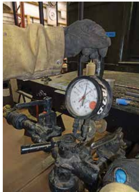
Charging the air lines and checking for correct pressure and leaks.
