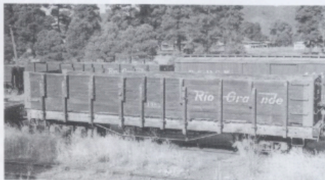
Gondola 1082 shows many extra holes, both in the original side sill where the double U-bolt stake pockets were removed, as well as the movement of the two end stakes inboard a few inches. Photograph taken at Chama on 9/15/1987. (Stan Rhine)
