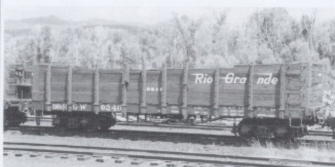
Gondola 9249 has its original size four board sides, as well as the one-piece corner irons. Photograph taken at Chama on 8/6/2001. (Stan Rhine)
