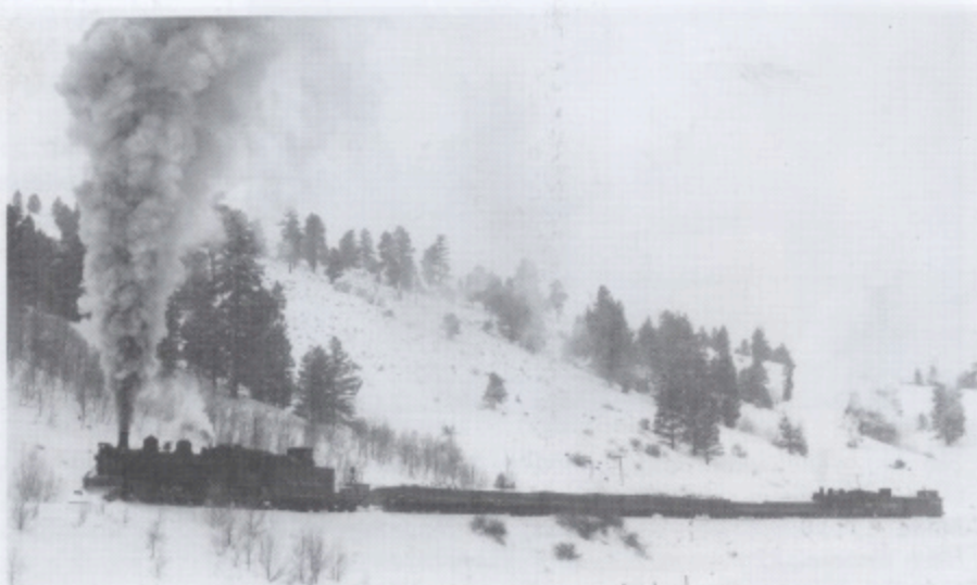
A freight train ascends Poncha Pass on January 28, 1949. The leading locomotive carries a snowplow and is followed by a flanger plow to clear the line where needed. Photo by Robert W. Richardson. Photo from the Richard L. Dorman Collection of Narrow Gauge Railroad Photographs , Friends of the Cumbres & Toltec Scenic Railroad. (Caption by Vern Glover)
