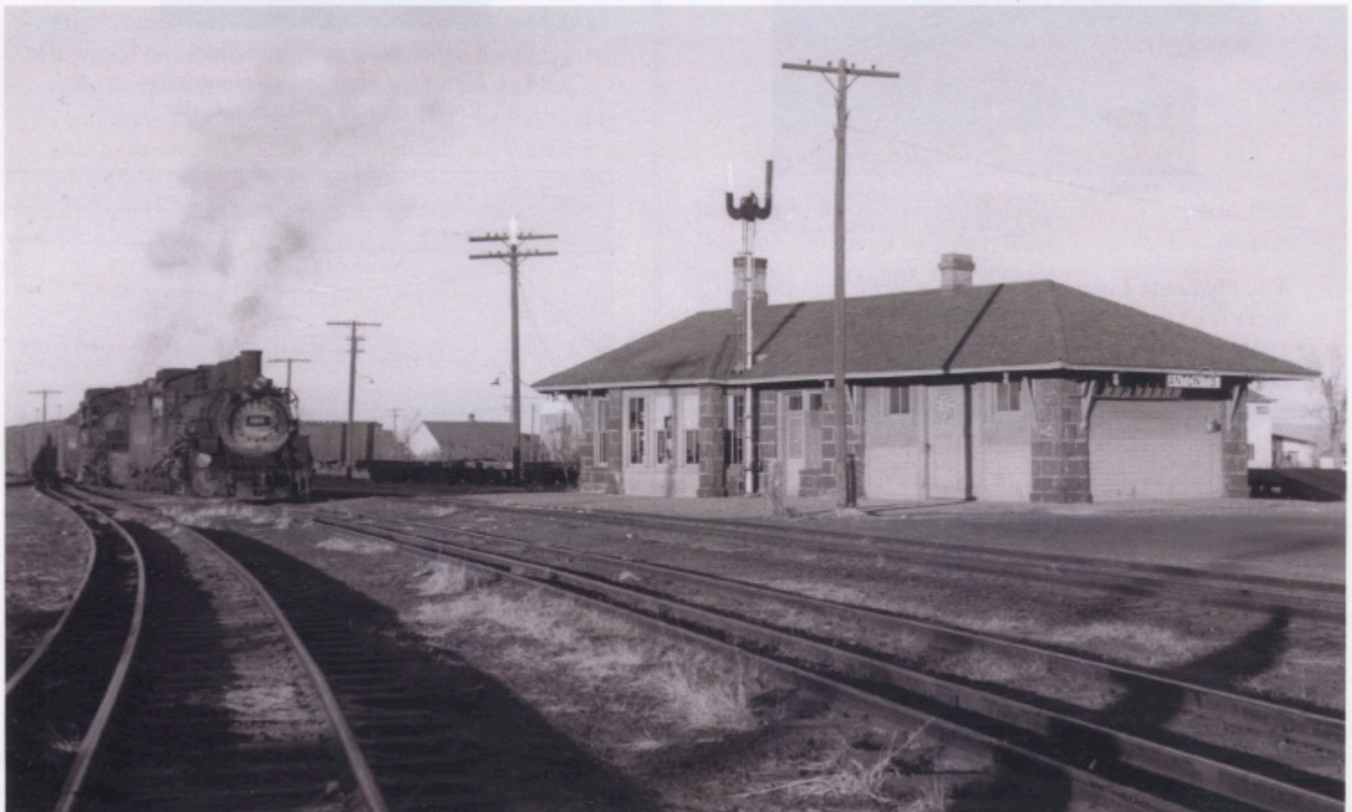
RD016-012 This Robert W. Richardson photograph shows K-37 #490 on the point of a double-headed westbound freight in Antonito, CO. Taken on January 1, 1958, note the dual-gauge track and the loading platform at the rear of the depot. Photo from the Richard L. Dorman Collection of Narrow Gauge Railroad Photographs, Friends of the Cumbres & Toltec Scenic Railroad, Inc.
