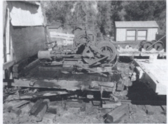
The double drum winch after being power-washed by Don Duell for most of one day. It actually cleaned up very well.
